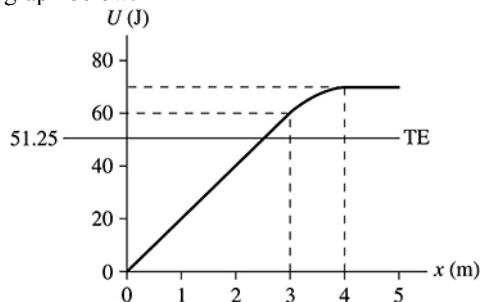
**(b)** Mechanical energy is  $E = K + U$ . From the graph,  $U = 20$  J at  $x = 1.0$  m.
